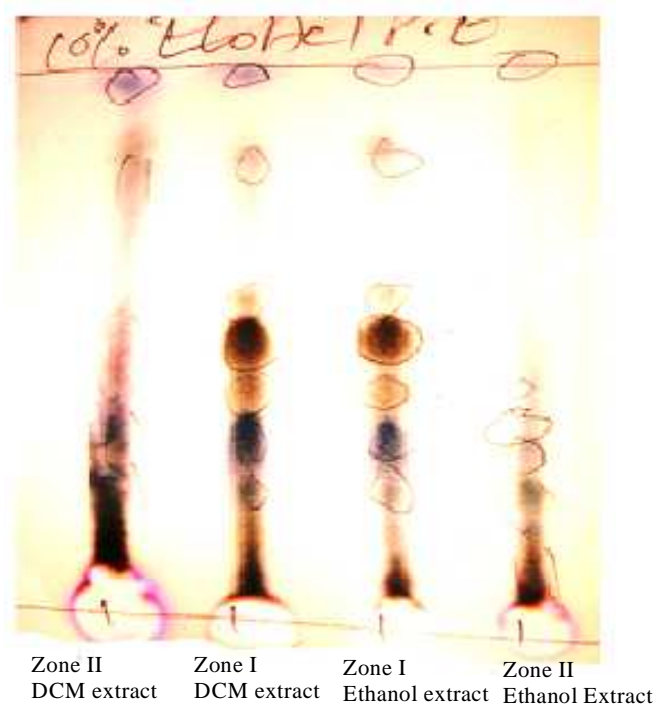
Figure 4: Thin Layer Chromatograph fingerprint of the compounds from the root barks of Harrisonia abyssiniaca from Zone I and Zone II.
