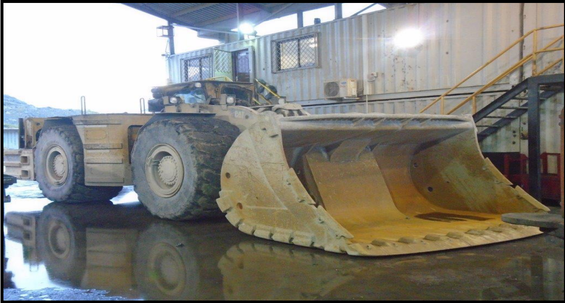
Figure 3.4: Bogger machine used for pushing materials and loading trucks underground.
