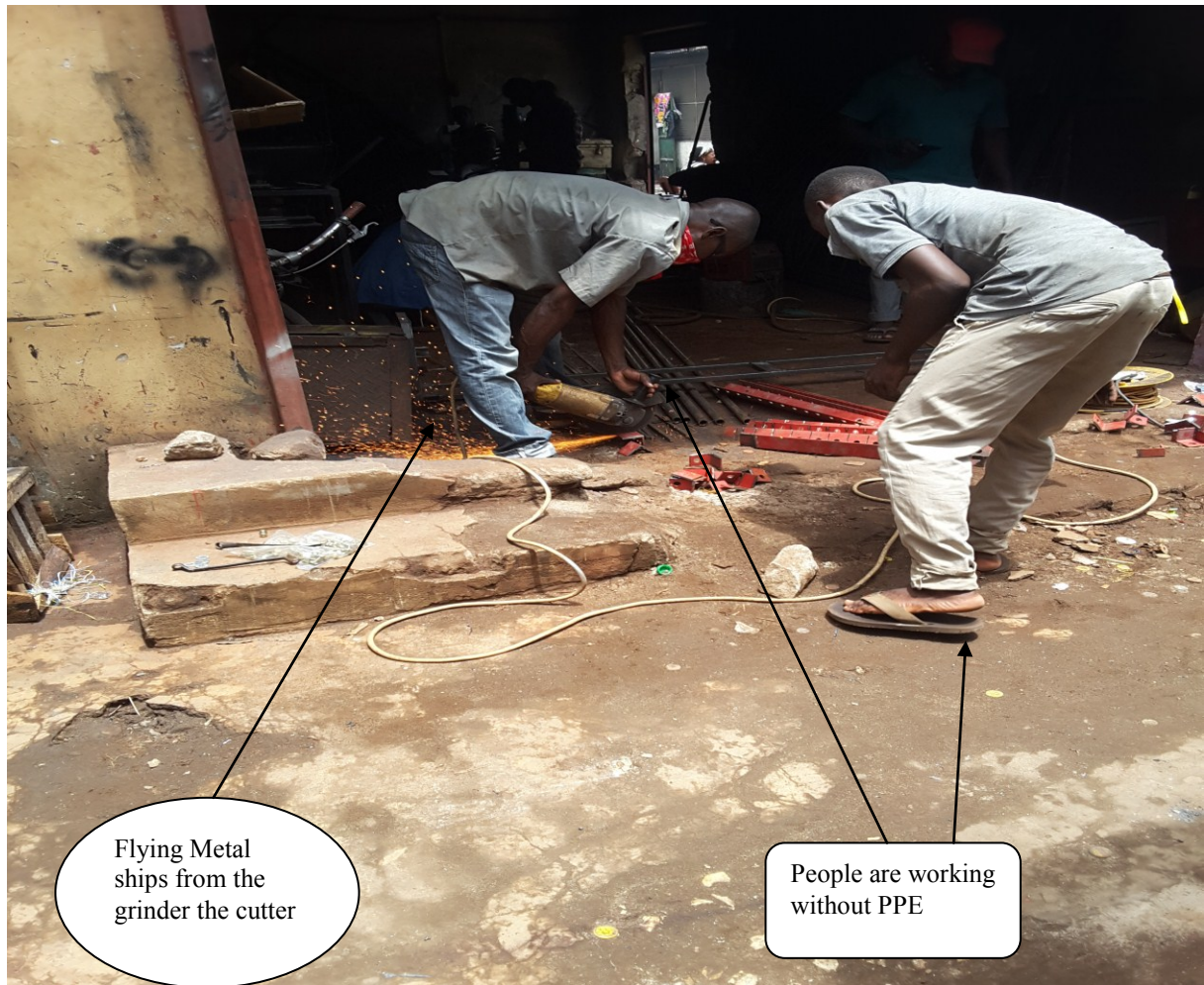
Figure 5: Some of the observed welders working without recommended PPEs in one of the workshops (Photo by a researcher)
